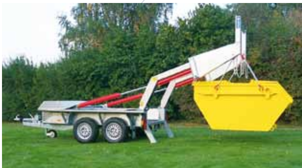
Deposit tipper trailer.
