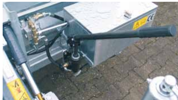
Electro-hydraulic pump with emergency hand pump.
