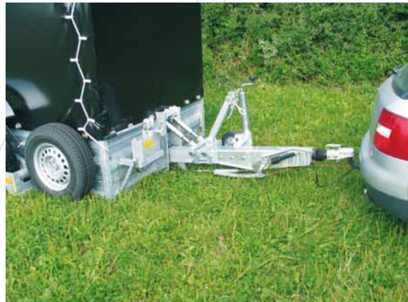
Trailer does not have to be unhitched for lowering.
