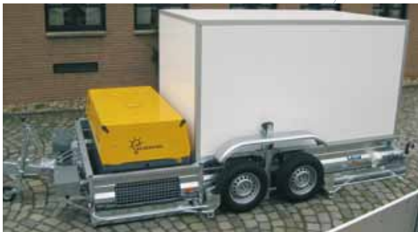
PT35 box body with generator for supplying power.
