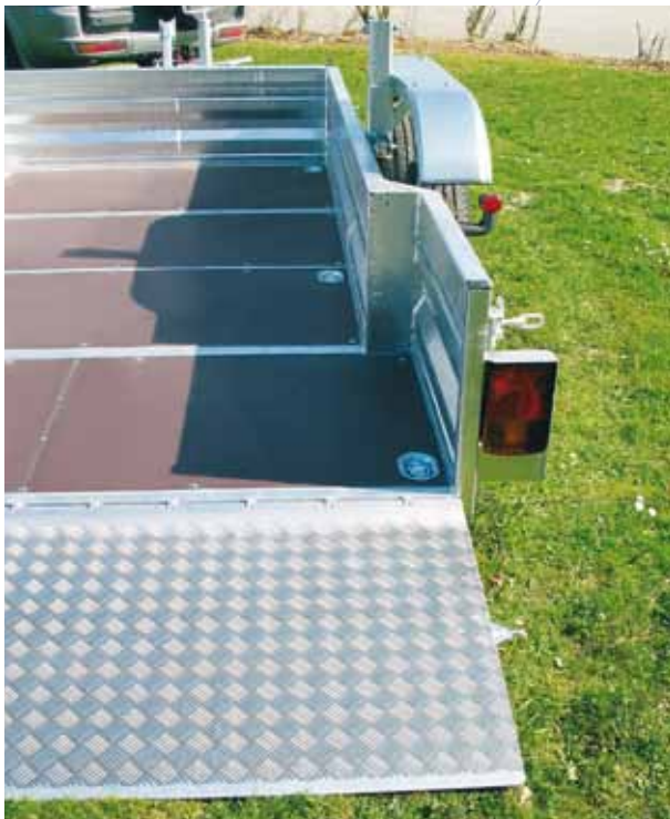
Trailer with wider side panels in the back and a longer loading ramp.
