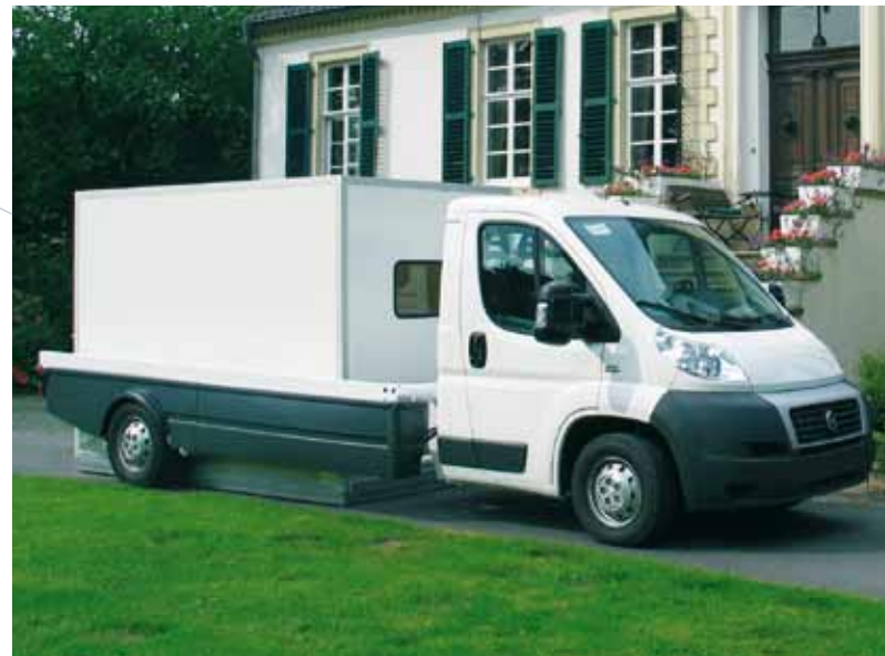
The Vario-Liner is lowered to the ground.
