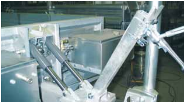
The locking lever is open at the front on the trailer hitch to lower the trailer.
