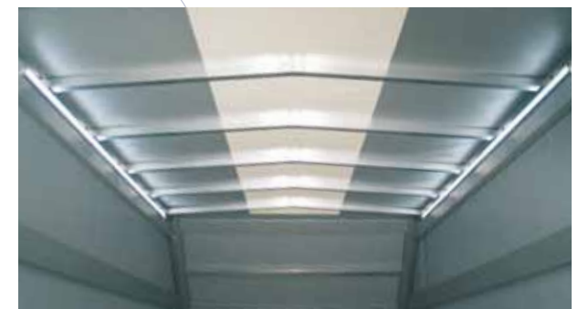
Interior LED lighting (12 or 24 Volt) for tarp frame and box bodies.
