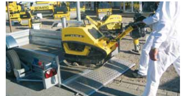
Loading a vibrating compactor.
