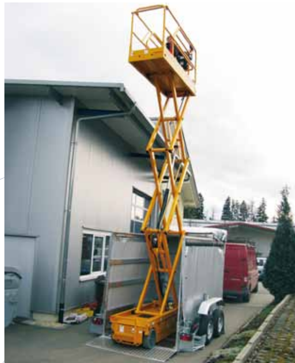
Thanks to the sliding tarp on top, you can raise a loaded lifting platform all the way to the top.
