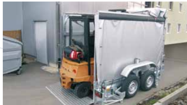
With the Miniliner sliding cover, the roof and side walls can be moved forward.
