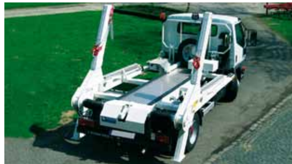
AKFV deposit tipper unit can be widened, up to 12 tons.
