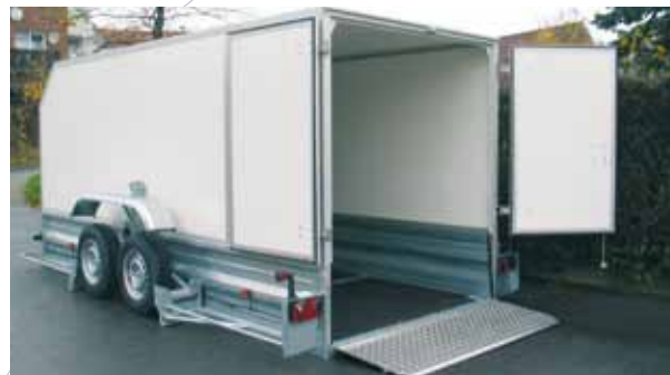
PT35 with box body, 2-rear wing doors, and tailgate lowered.
