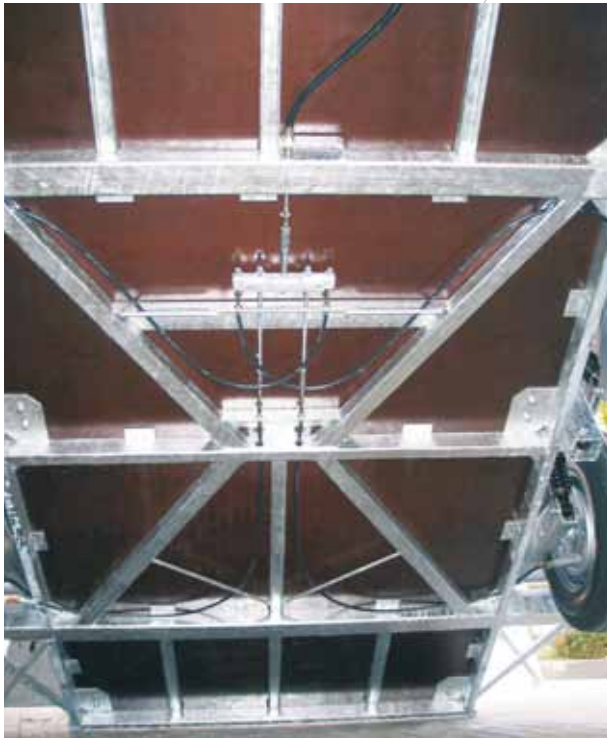
Bottom frame of the PT35 with multiplex wood panels.
