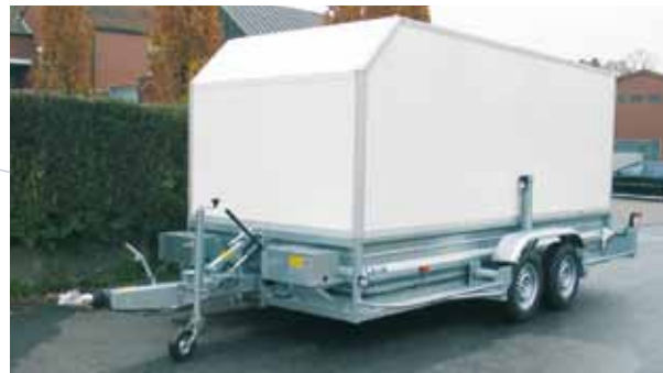
PT35 with box body and with a with 45° angle in front in driving position.
