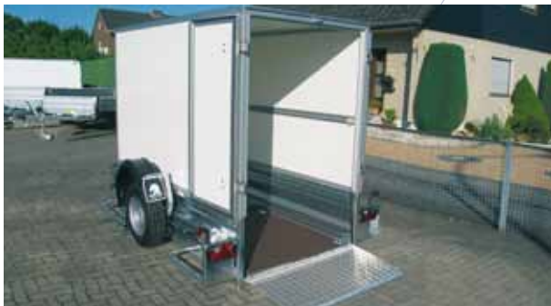
The PT18 with box body and 2-wing rear door.
