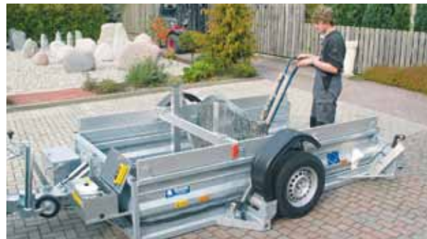
The locking bar can be moved anywhere along the entire length of the trailer.
