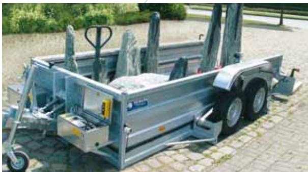
Goods must be tightly and securely lashed to avoid potential hazards. Lashing rings built into the bed.
