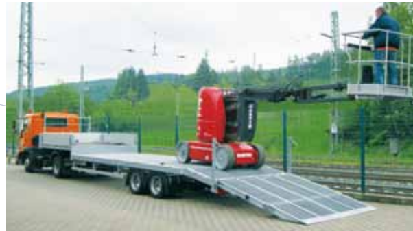
City semi-trailer with a total weight of up to 14 tons.
