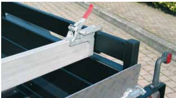
Raised side panel for partition bar.
