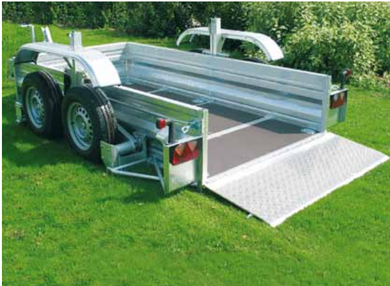
PT35 lowered down to the ground.
