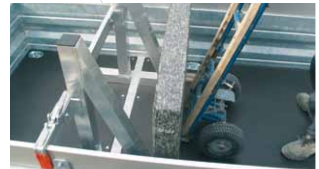
Support rail for transporting stone with a locking bar.
