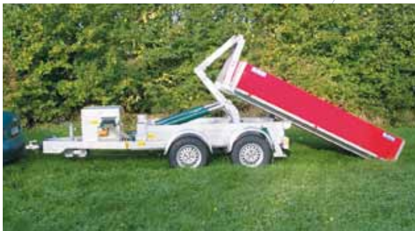
Roller tipper trailer.
