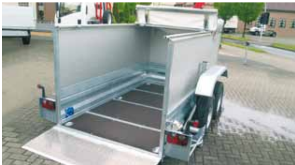
Raised side panels made of aluminum with sliding tarp.
