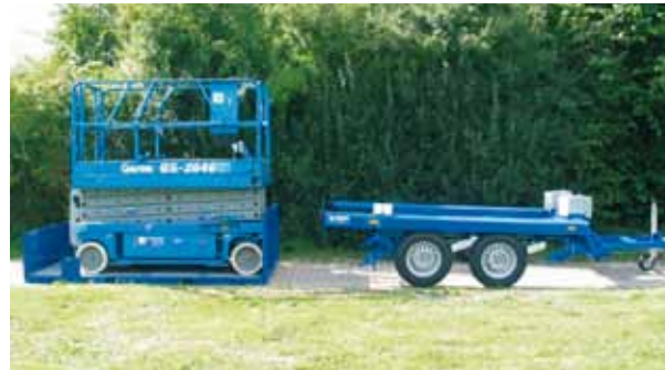
The platform of the trailer can be parked and stay on-site with the goods.
