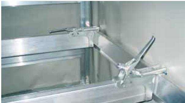
Partition bar for clamping to the tarp frame.
