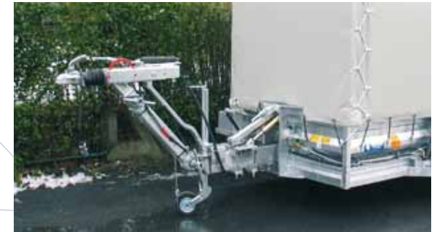
Height adjustable drawbar, coupling height max. 1100 mm.
