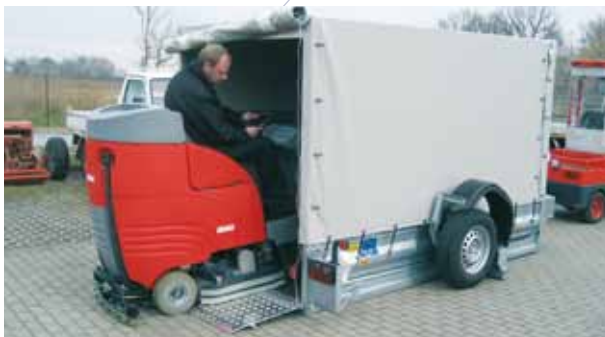
When loading a cleaning machine, no damage to suction scrub brushes and guards.
