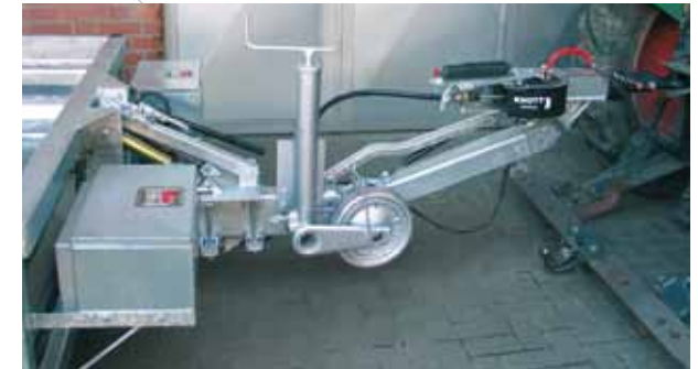
Height adjustable drawbar with DIN towing eye and reinforced support wheel.
