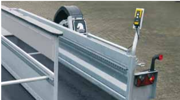
Control unit for the electric pump on the rear.
